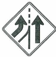
LEFT ADDED LANE
